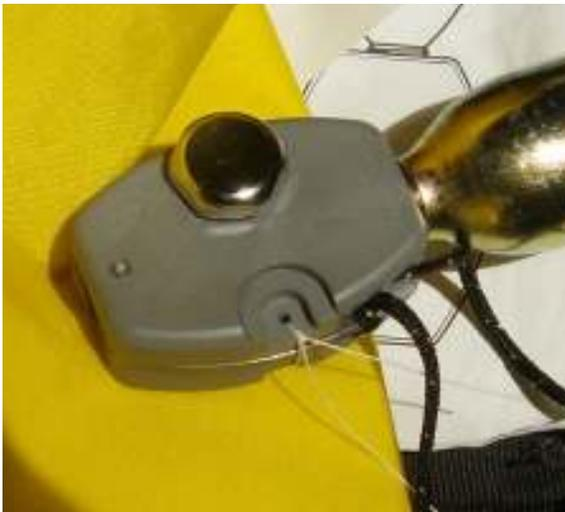
Figure 7. Oral Inflation Valve Thumb Screw
