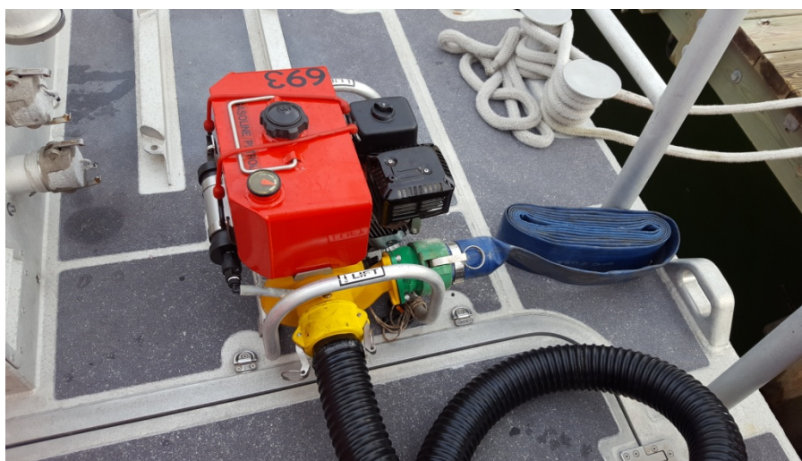
Figure 5-6 Drop Pump Readied for Dewatering Action
