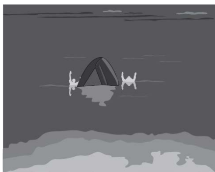
Figure 2-3 White Hot Thermal Display
