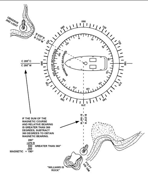
Figure 3-48 Converting Relative Bearings to Magnetic; Sums Greater than 360°
