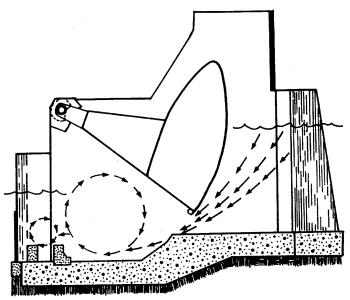
Figure 3-85 Roller Gate Dam
