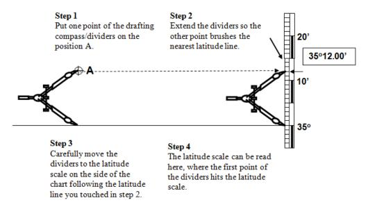
Figure 3-50 Finding Latitude of a Position
