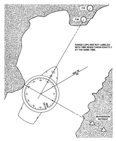
Figure 3-64 Visual Fix Using Terrestrial Ranges
