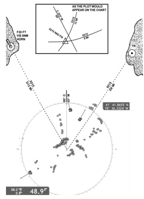
Figure 3-61 Obtaining a Radar Fix Using VRM
