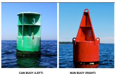
Figure 2-2 Can and Nun Buoys, "When Returning From Sea"
