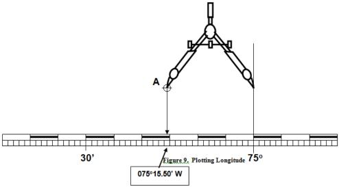
Figure 3-52 Finding the Longitude of a Position
