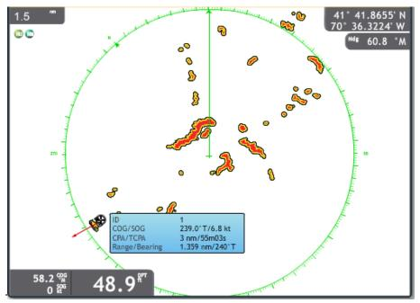
Figure 3-30 Automatic Radar Plotting Aid (ARPA)
