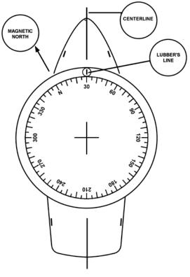
Figure 3-38 Lubber's Line and Magnetic North
