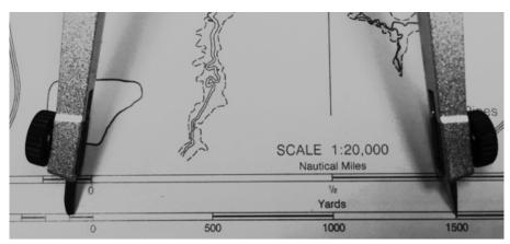
Figure 3-58 Graphic Scale Distance Measurement
