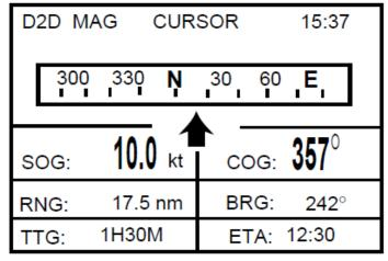
Figure 3-36 Heading Sensor Data Shown on GPS Display
