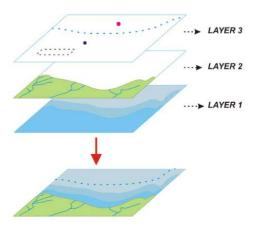
Figure 3-18 Electronic Chart Overlays
