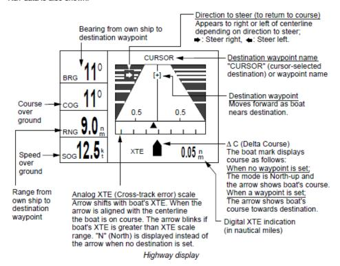
Figure 3-76 GPS Highway Display
