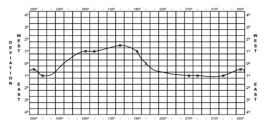
Figure 3-44 Example Deviation Curve
