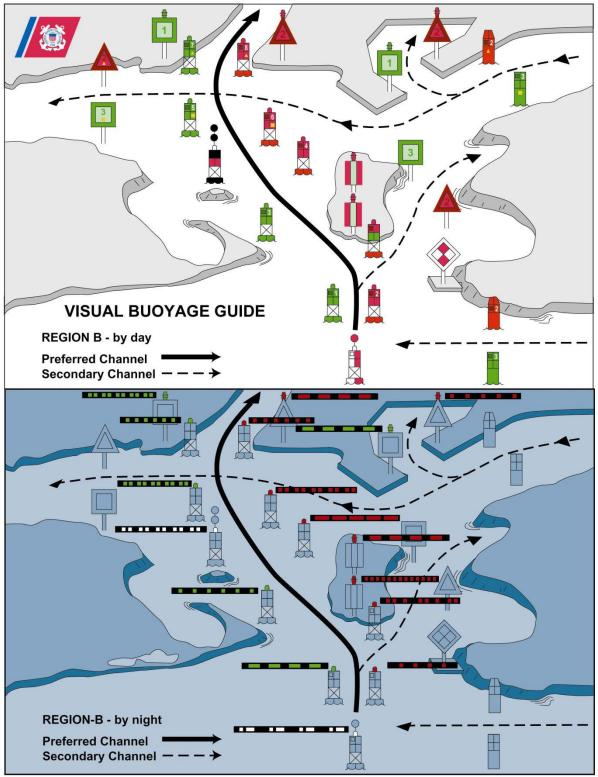
Figure 2-12 Visual Buoyage Guide
