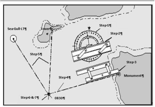
Figure 3-62 Obtaining Radar Fix Using EBL
