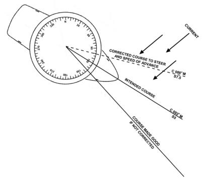
Figure 3-83 Compensating for Set and Drift
