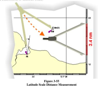
When the distance being measured is greater than the span of the dividers, the dividers can be set at a certain distance. Take the known distance and starting at the first point continue marking on
