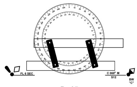
Figure 3-69 Laying Trackline
