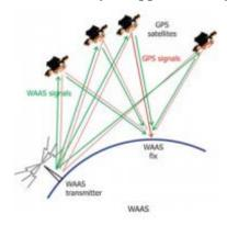
Figure 3-24 Wide Area Augmentation System (WAAS)
