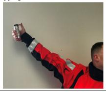
WARNING 🎇 Prior to pulling lever downward, position all fingers below top of signal.
