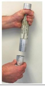
Point the ejection end of the signal (the end opposite the red knurled band) away from personnel, equipment, and materials. Slowly push the cap onto the primer (red band) end until the cap meets the edge of the knurled band. DO NOT PERMIT THE CAP TO GO BEYOND THE RED BAND.
