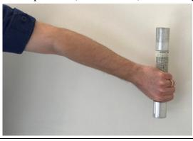
Strike the firing cap bottom sharply with the palm of the right hand, keeping the left arm rigid and pointing straight up.
