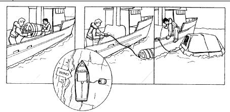
Figure 4-1 Manual Deployment of Survival Raft
